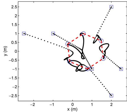
Fig. 6. Hexagonal formation trajectory for SMC-based control scheme [10].
