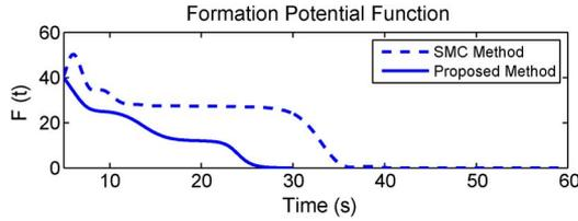
Fig. 7. Formation potential function decrement comparison between SMC-based control scheme [10] and the proposed control method.
