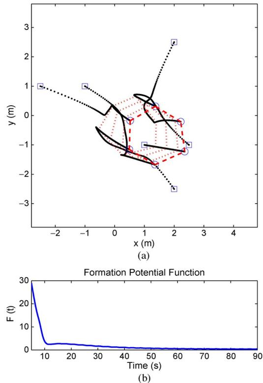
Fig. 5. Moving hexagonal formation while tracking the leader. (a) Formation trajectory. (b) Formation potential.
