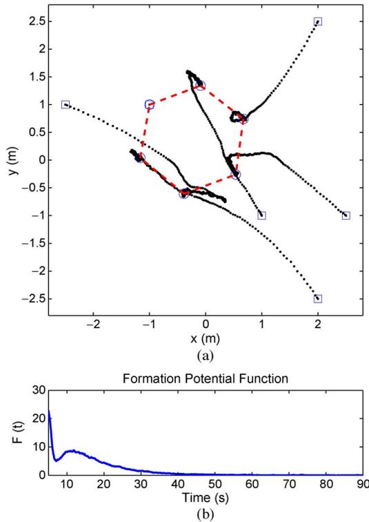
Fig. 4. Hexagonal formation in the presence of 20-dB noise and one agent failure. (a) Formation trajectory. (b) Formation potential.
