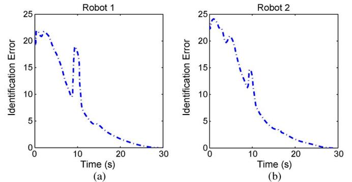
Fig. 3. Identification error during formation control. (a) Identification error of the first robot. (b) Identification error of the second robot.
