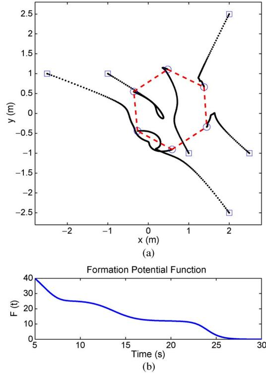
Fig. 2. Hexagonal formation of six agents with partially unknown dynamics. (a) Formation trajectory. (b) Formation potential.
