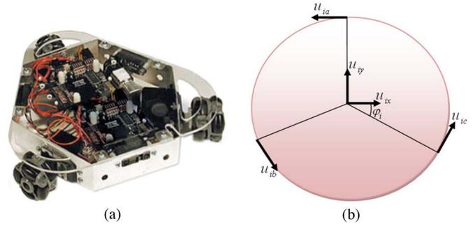
Fig. 9. PPRK platform used for experimental verification. (a) Real photograph. (b) Physical model.
